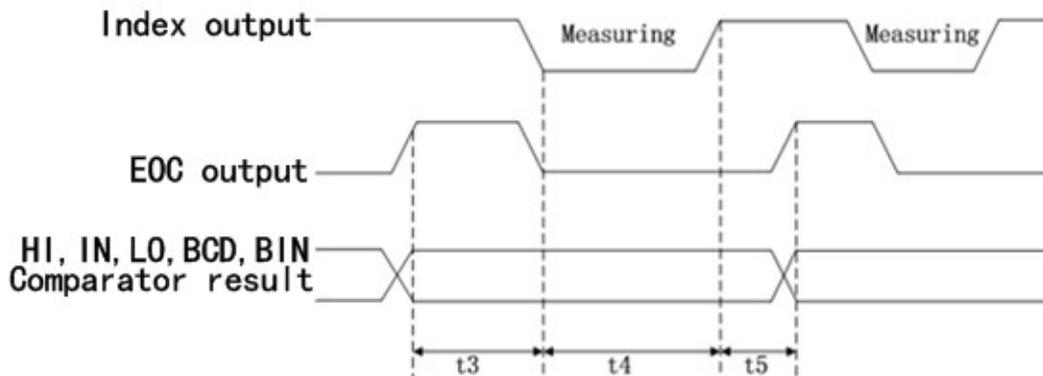
Figure 59 Internal Trigger Timing
