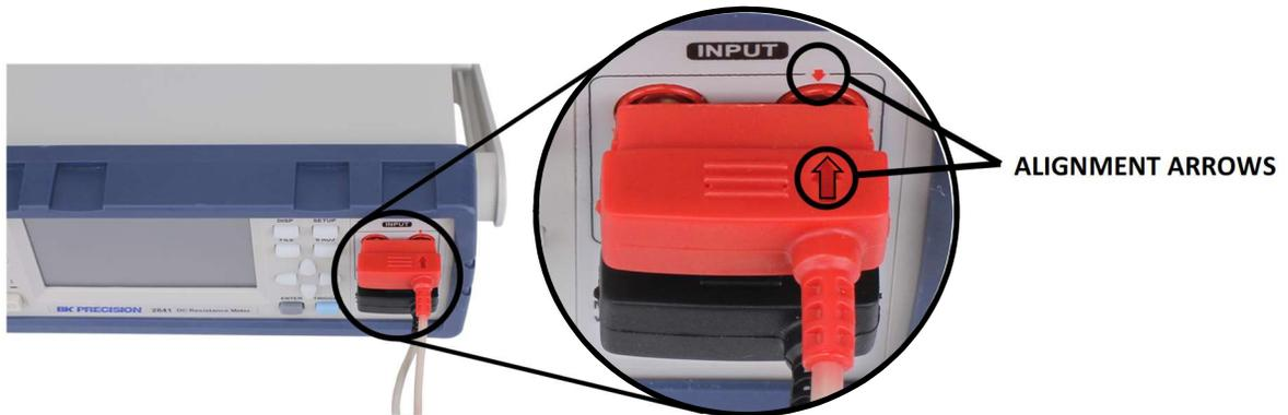
Figure 8 - Connection Alignment
