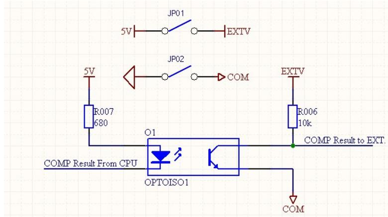
External control input circuit is shown as follows:
