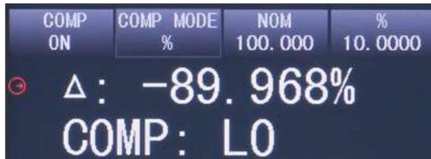
Figure 50 Comparator Display Percent Error
