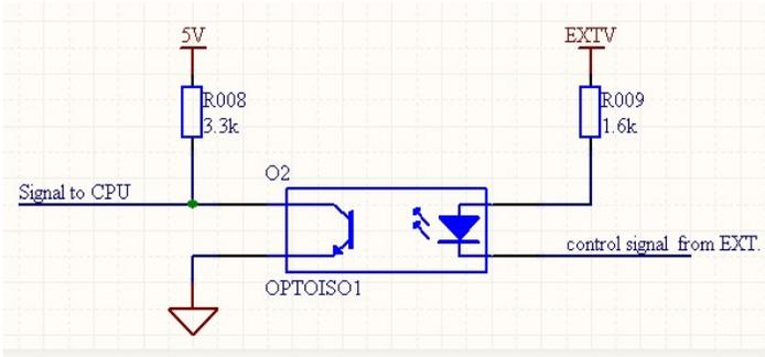
Figure 33 - Input Circuit
