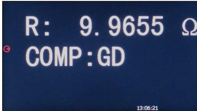
Figure 49 Comparator Display Enlarged
