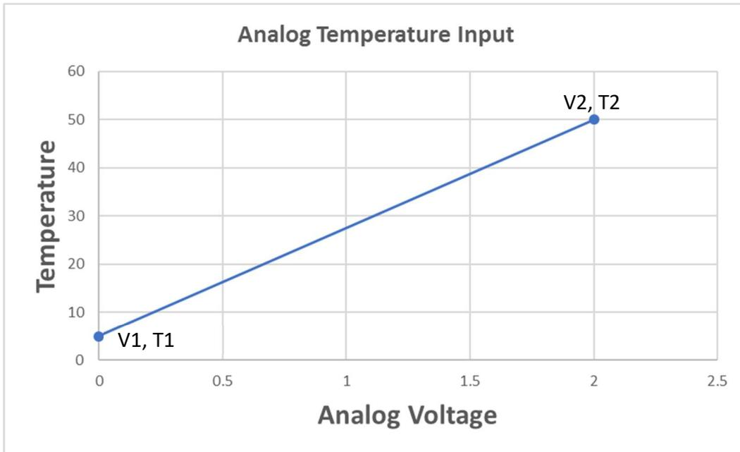
Figure 55 - Analog Input Voltage vs Temperature
