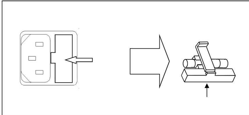
Figure 39 - Replacing Fuse
