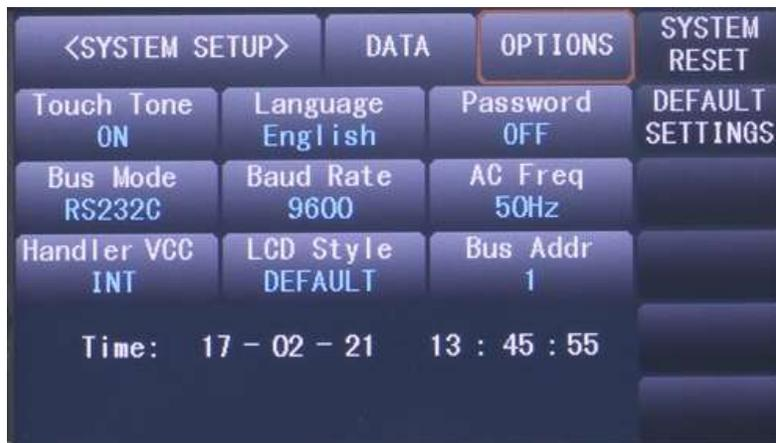
Figure 28 - System Setup
